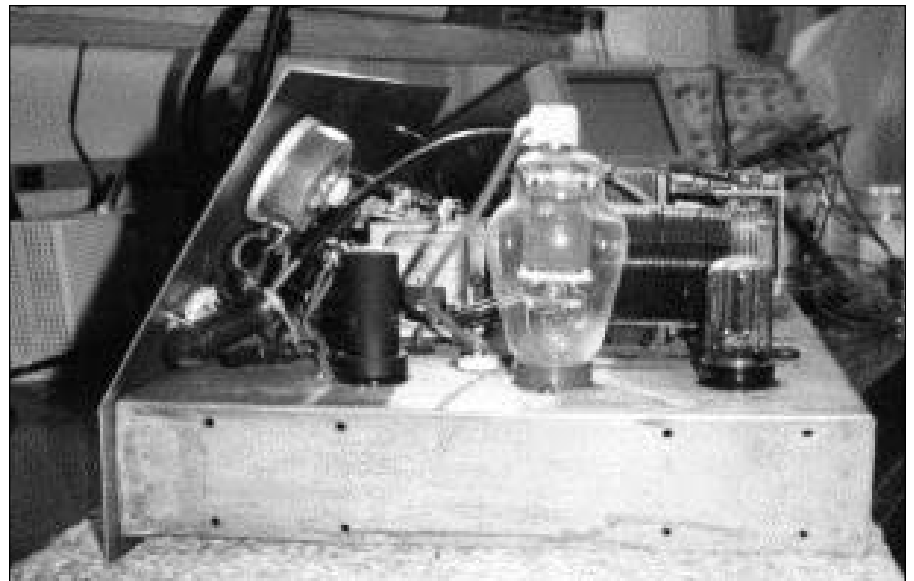
Original Rife beam ray unit of about 25 watts power; uses 809 output tube.
